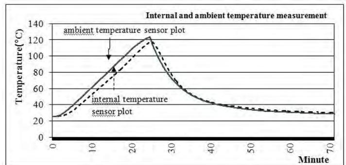
**Figure 7.** Time-dependent change graph of values collected from internal temperature and ambient temperature sensors
