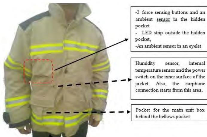
Figure 5 The placement of the electronic system
