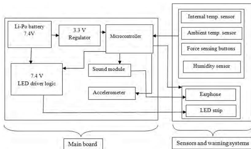
Figure 1 Blockdiagram of electronic system
