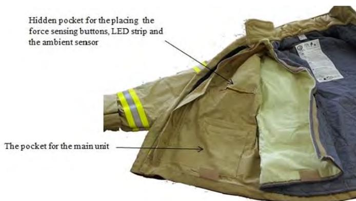
Figure 3 The hidden pocket and the pocket of the main unit
