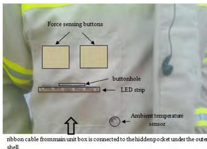
Figure 6 Electronic equipment in hidden pockets
