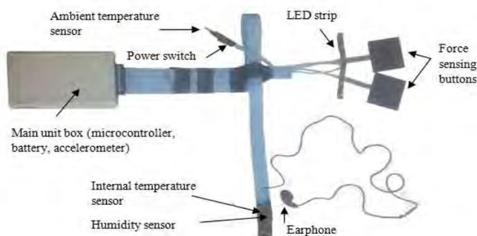
Figure 4 The electronic circuit
