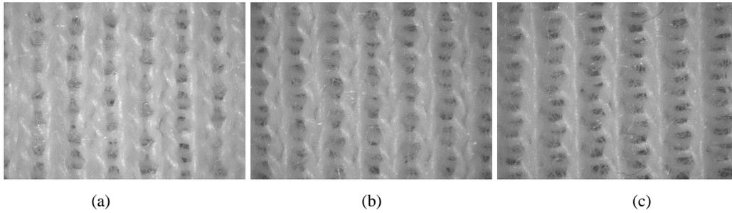
**Figure 6.** Photos of the samples (a) full plating, (b) half plating, (c) without elastane
