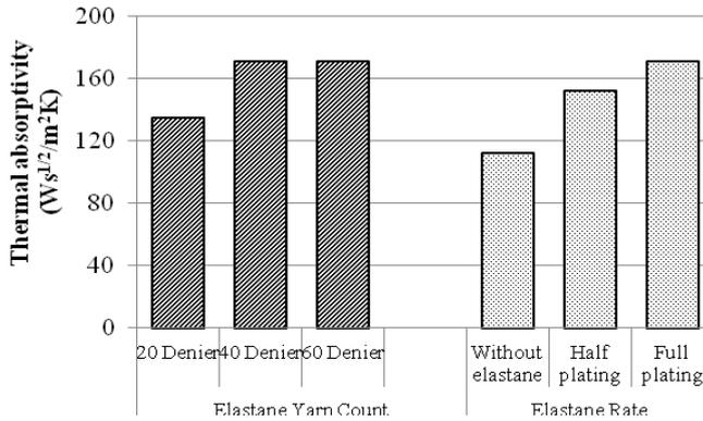
Figure 9. Thermal absorptivity results
