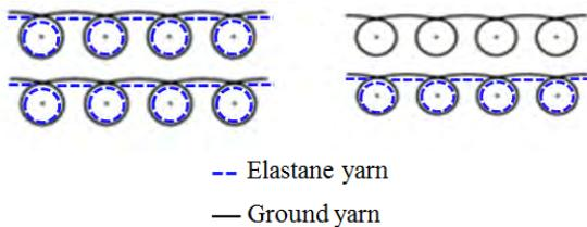
**Figure 1.** Needle diagram of the elastic single jersey fabrics: (a) in every courses (full plating), (b) in alternating courses (half plating) [4]
